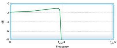
Figure 12: Frequency magnitude response of a decimate-by-2 compensation FIR filter View full-sized image
