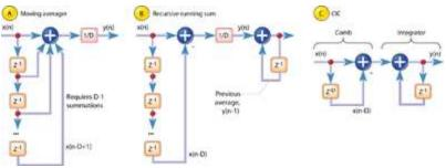
Figure 2: D-point averaging filters View full-sized image
