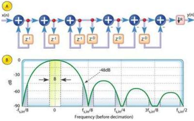
Figure 8: 3rd-order CIC decimation filter structure, and magnitude response before decimation when D = R = 8
