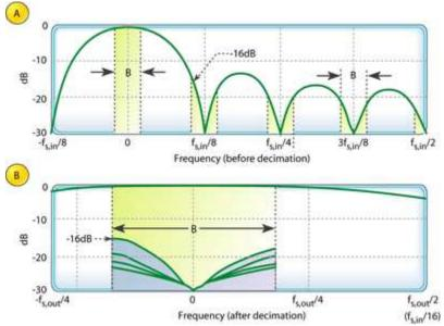
Figure 6: Magnitude response of a 1st-order, D=8, decimating CIC filter: before decimation; aliasiing after R=8 decimation
